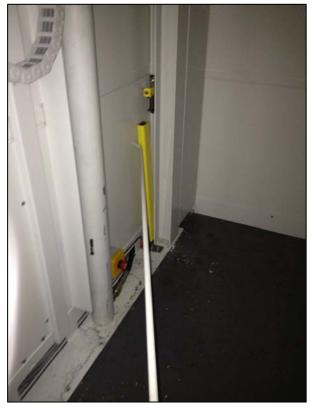
6. Place rod back in holster making sure it butts-up to the back stop. Please note the rod locates in one plane only, this is to ensure the rod doesn't fowl the underside of the platform.
